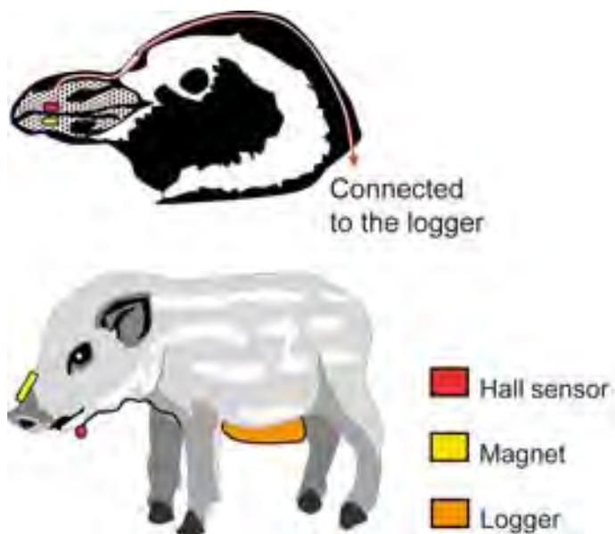
**Figure 1:** Schematic representation of the jaw movement recorder on a gentoo penguin *Pygoscelis papua* (top) and a young wild boar *Sus scrofa* (bottom). A magnet and a Hall sensor, sensitive to the strength of the magnetic field are placed on the two mandibles, facing each other. When the mouth opens the Hall sensor senses a reduction in the intensity of the magnetic field and sends this information via a cable to the bio-logger attached on the body.
